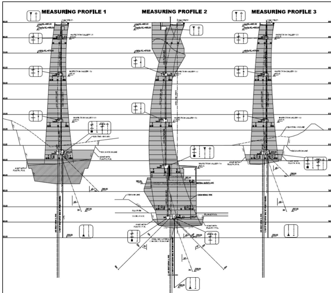
Figure 2: Typical Instrumentation profiles
