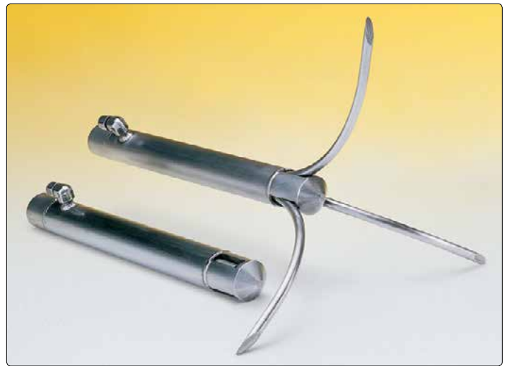
● Single-action borros anchor before and after prong extension.
