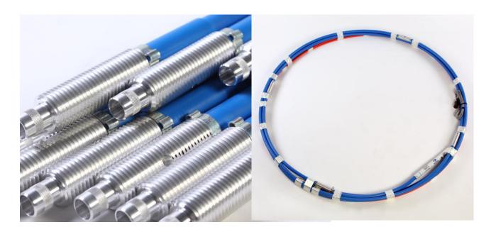
Lightweight and flexible, our pre-assembled Multi-Point Borehole Extensometer (MPBX) is a six anchor points with an integrated electronic readout head. The small instrument diameter means that the head can be recessed in a 50 mm (2 inch) borehole - no need for oversize holes or reamed collars. It also allows multiple MPBX's to be installed in the same long borehole.
