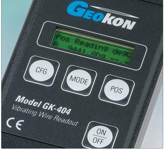
• Close-up of the Model GK-404 Vibrating Wire Readout control panel and LCD display.
