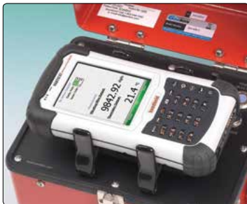
• Live Readings screen shot, displaying vibrating wire strain gage data.
