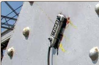
• Model ST-350 attached to steel truss.
