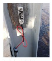
Installation of a Strain Gauge
