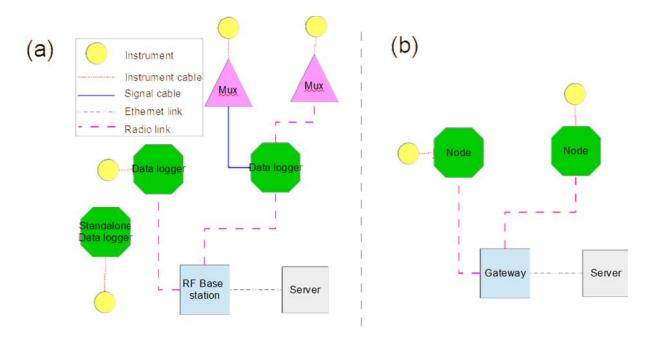
Figure 4 (a) Schematics of the of the network topology of the system deployed at the Meadowbank mine (b) Schematics of the network topology at the Lake Bloom mine
