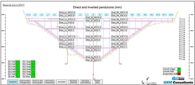
Figure 9: Virtual Mimic screen showing Pendulum measurements and location
