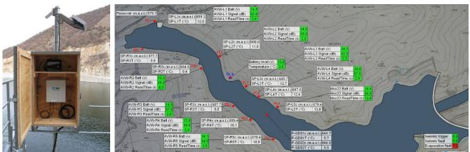
Figure 5: Remote open standpipe monitoring
