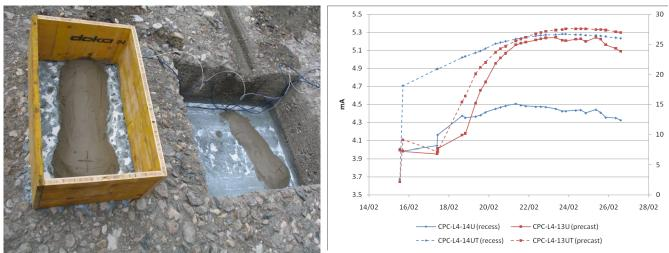
Figure 4: View and graph of precast and recessed total pressure cell installation methods test.
