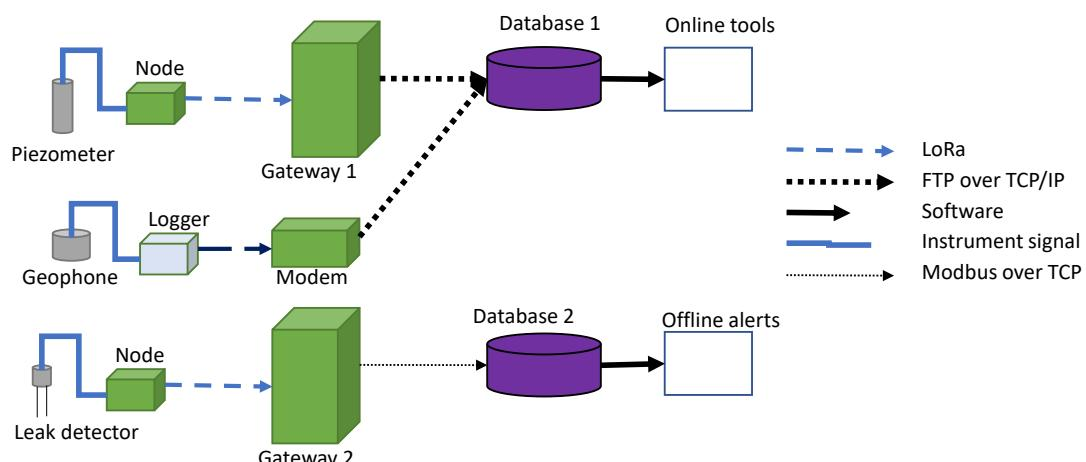
Figure 3 Comparison of the architectures of three separate IoT schemes used on a single gold mine's TSF
