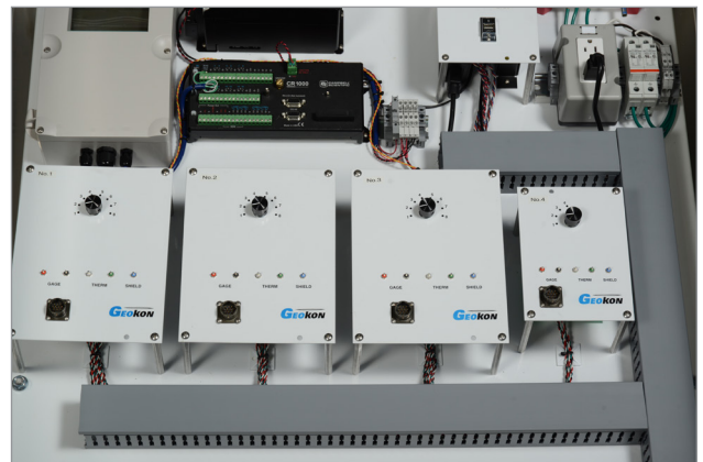
DL Multiplexers and manual switch
