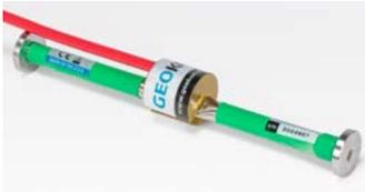
Model 4200-7 Extended Range (10,000 µε) Strain Gauge.
