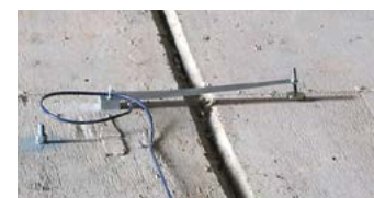
Model 4420-3 Low Profile Crackmeter for measurements in the "Z" direction.
