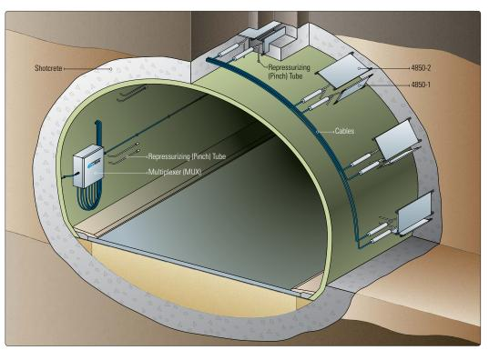
• Illustration shows typical installation in tunnel lining.
