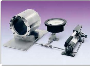
● Model 5075 Biaxial Modulus Chamber.
