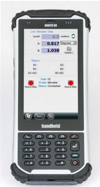
Model FPC-2 Field PC showing a Live Tiltmeter Data reading screen shot.
