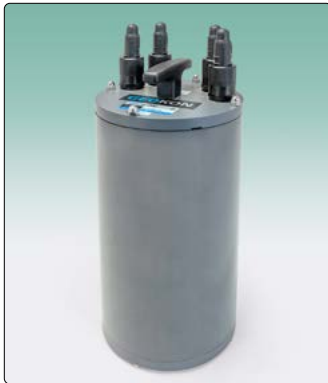
● Model 8002-WP-4 (LC-2x4WP) Waterproof Four-Channel Datalogger.
