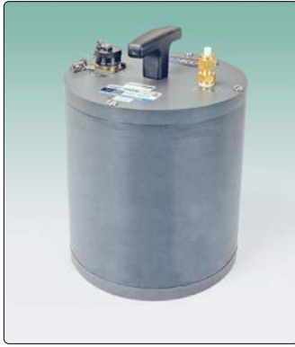
● Model 8002-WP-2 (LC-2WP) Waterproof Single-Channel Datalogger.
