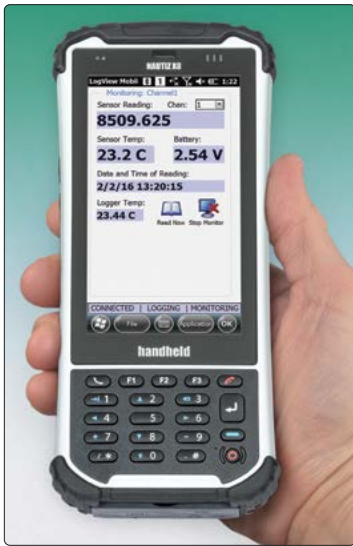
● Model FPC-2 showing LogView Mobile Datalogging and Monitoring screen.
