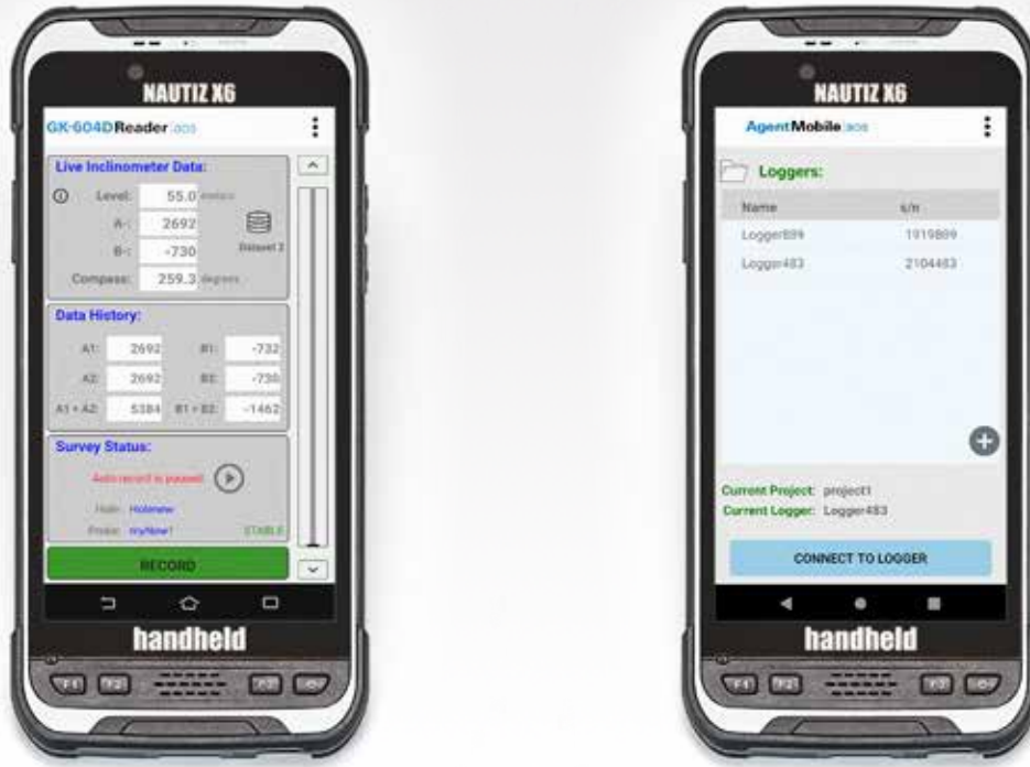
Model FPC-3 Field PC running GEOKON Applications GK-604D Reader (left) and Agent Mobile (right).
