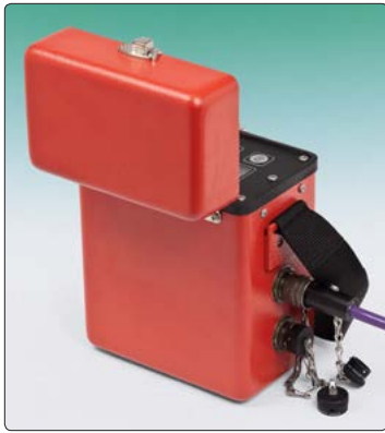
● Model GK-502 Load Cell Readout, showing load cell and communication connectors.
