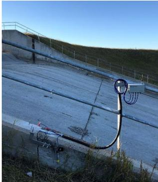
Crack monitoring on the spillway chute
