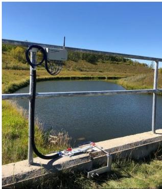
Crack monitoring on the spillway wall
