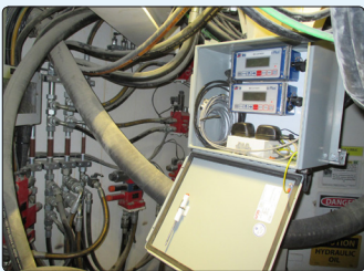
• Ground vibration measurement with Instantel geophones installed on the Boring machine structure and in the frozen soils
