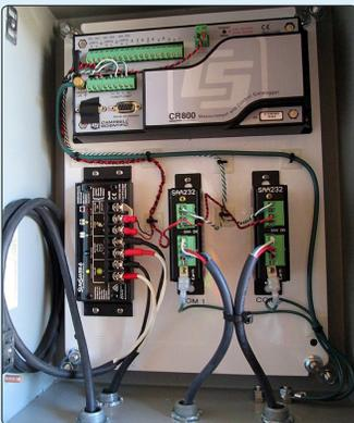
• Solar powered data acquisition system for SAA
