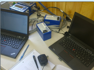
• Seismographs and datalogger system for remote monitoring of vibrations and crack openings
